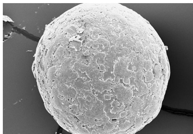
Fig. 1: SEM of insulin microspheres containing drug/polymer ratio 1:15.6 ( F_2 ) at 500 \times magnification.
